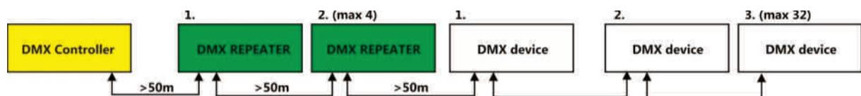
**Due to the bidirectional communication mode, it is not possible to install one DMX device between the controller and the splitter.** If a very long cable used in the system, more Repeaters can be connected (maximum 4), one after the other.
